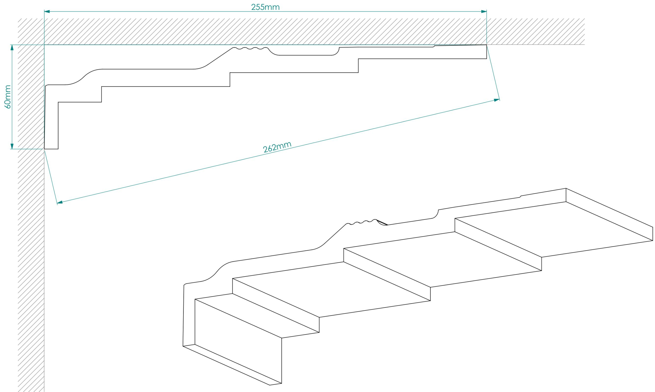
Manufacturing tolerance : refer to technical datasheet
