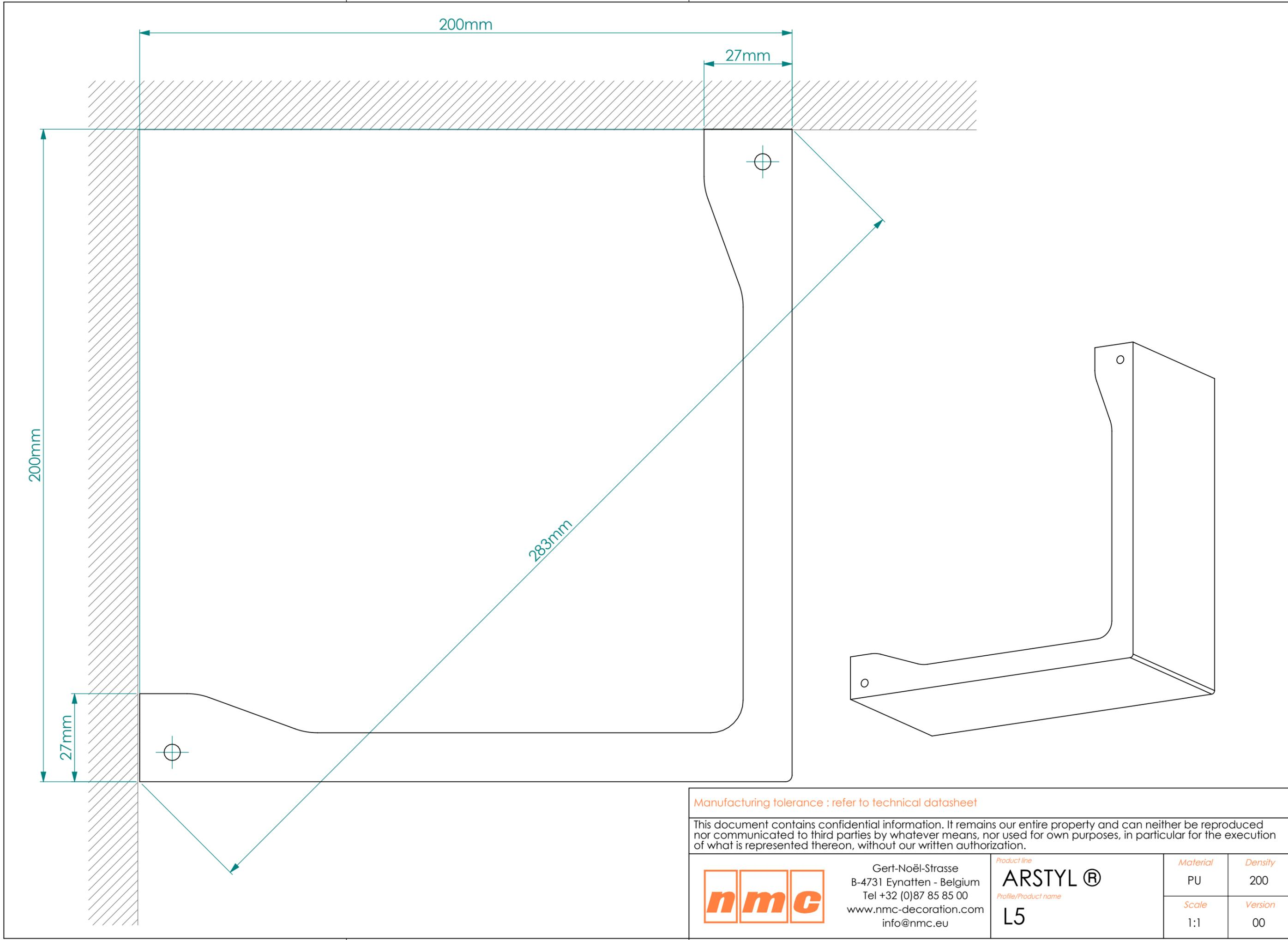
Manufacturing tolerance : refer to technical datasheet
