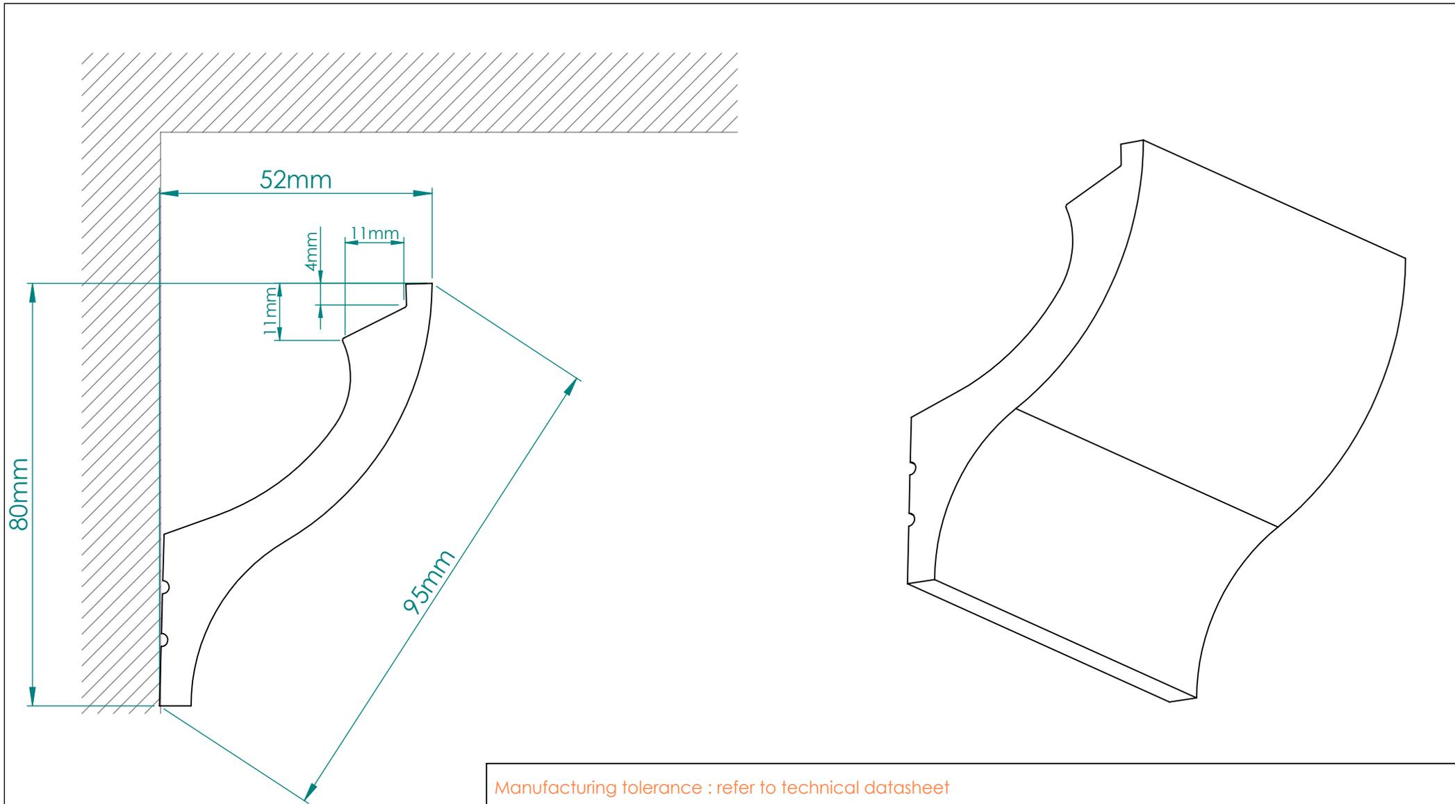
Manufacturing tolerance : refer to technical datasheet
